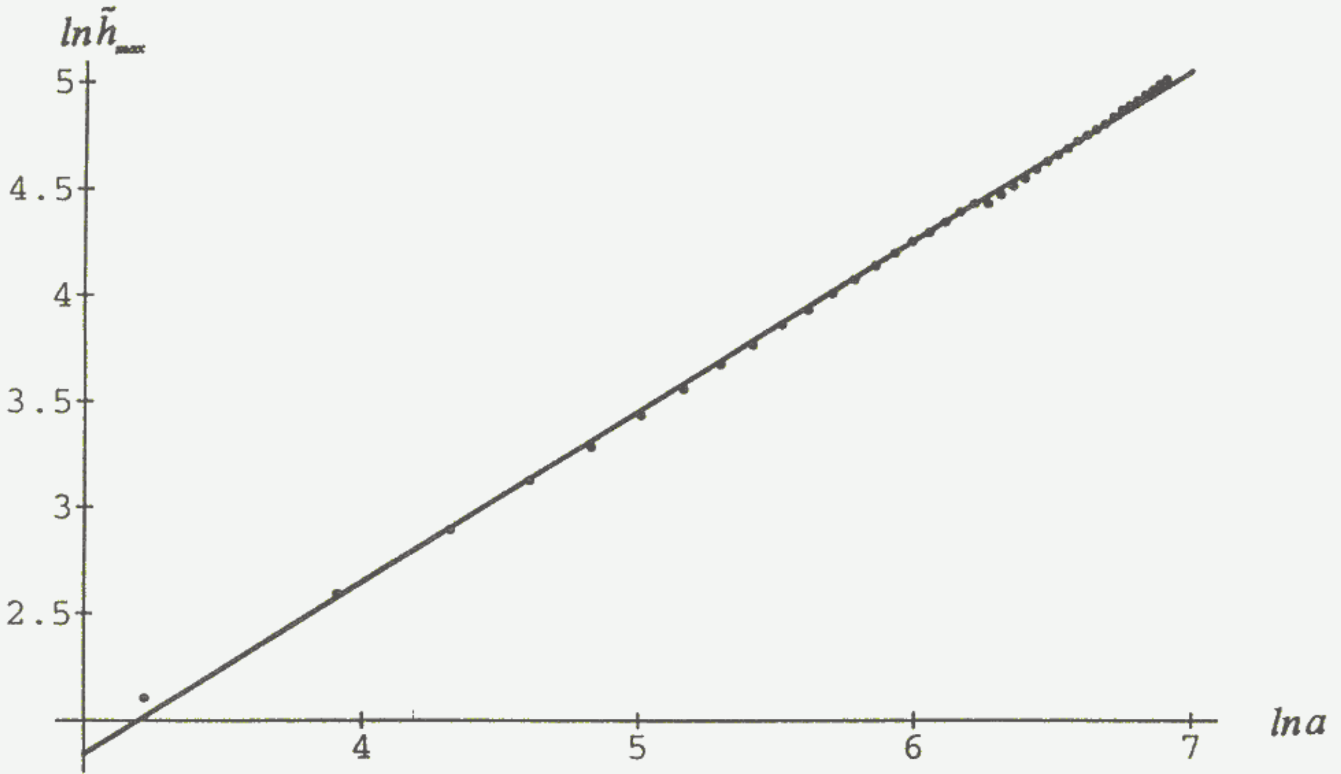
Fig. 4. Scaling law of the maximal height of ascension \tilde{h}_{\max} versus the capillarity a .
